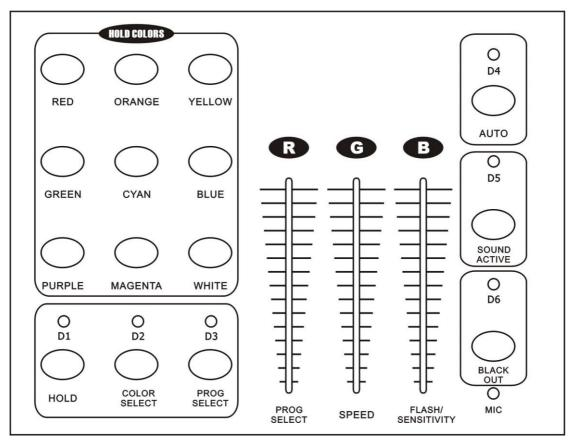
D1, D5 is Red LED, D2, D4 is Green LED, D3, D6 is Yellow LED.
