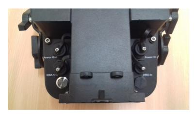
The Battery switch (Silver button) will connect or disconnect the batteries from the fixture, this helps extend the battery life.
