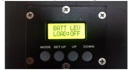
Once the display shows BATT LEV use the SET UP button to obtain LOAD: OFF (as shown above), then press the UP or DOWN keys so the display show LOAD: ON, the unit will now be ready to operate.
