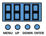
Switch on the unit and the display will show **rESt**, this will reset the unit to the start point which will show **A001**.
